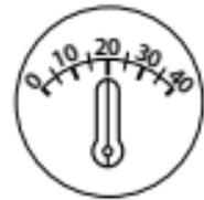
**Power Reserve:** found on automatic watches, this 0 zone displays the hours of autonomy remaining of a movement after it has reached its winding peak.
